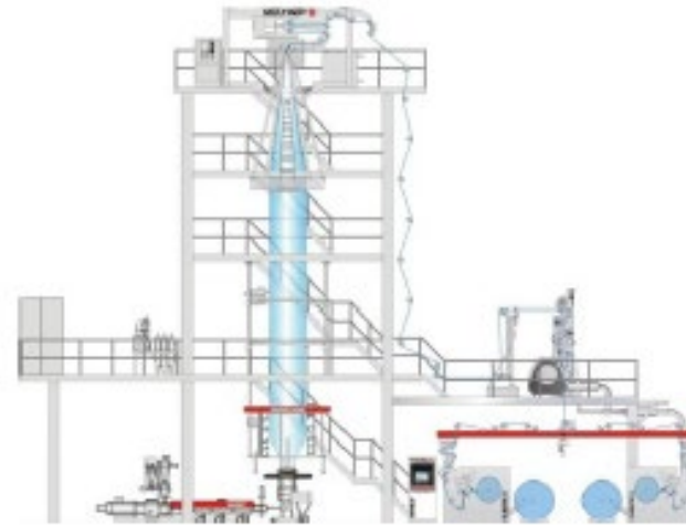
Direct processing of regranulate to 2 nd blown film
